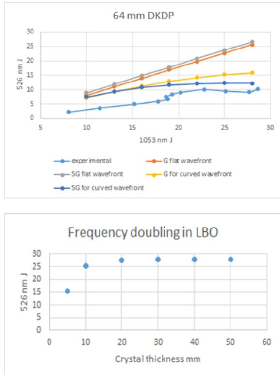
Figure 5: Experimental and simulated conversion efficiencies obtained in thick DKDP and LBO for 28J
